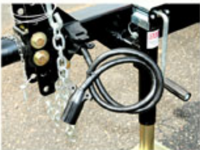
Removable trailer wiring harness prevents damage on the job site.
