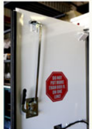
Redesigned double-wall doors with more industrial latches.
