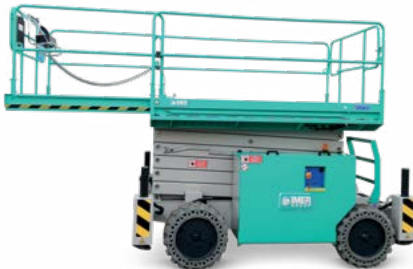
Manual deck extension of 59" (1.5 m) for a total length of 13' 8" (4.2 m)
