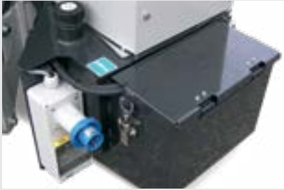
Thermal-magnetic switch panel and power line inlet.
