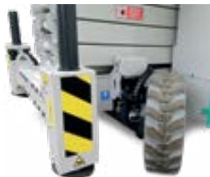
Reduced steering angle - 70° wheel inclination
