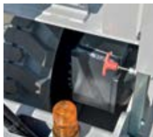
Standard manual emergency lowering device
