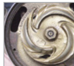
Competitor Impeller is effectively worn out.
