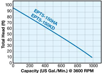
\* Convert to PSI , divide by 2.31 • Liquid-Water specific gravity 1.0
