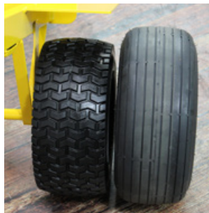
15" flat free tire option shown on left compared to standard 16" pneumatic tire.
