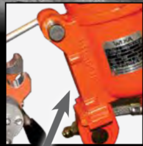
Integrated motor mount for Weka DK22F and DK32F only
