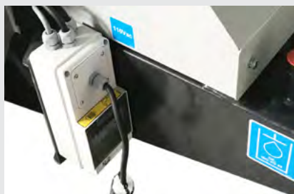
Thermal-magnetic switch panel and power line inlet.
