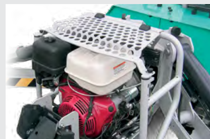
Rugged engine guard for improved protection.
