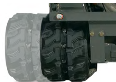
Hydraulically adjust the track width for added stability and traction.
