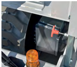
Standard manual emergency lowering device
