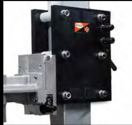
M-6 Heavy Duty Roller Carriage With cam lock quick disconnect 1:1 and 1:2 rack & pinion design and roller adjusters (included with M-6 stand only)
