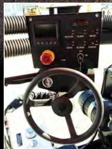
Digital Engine Panel, Fuel Gauge and E-Stop
