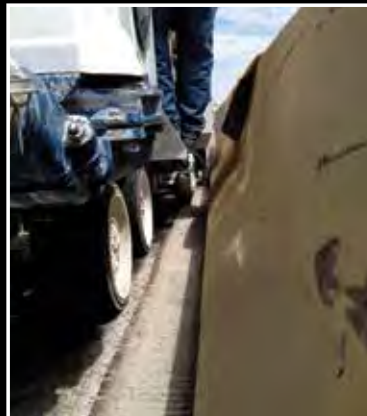
Ability to grind close to barrier walls and curb
