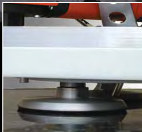
One of three 5" grinding platens (Velcro® surface)
