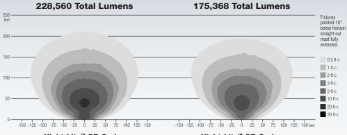
Night-Lite™ GR-Series 4 - 350W LED Light Output Area Lit to 0.5 Foot Candle (ft-c) or Higher: 45,010 ft² Night-Lite<sup>™</sup> GR-Series 4 - 250W LED Light Output Area Lit to 0.5 Foot Candle (ft-c) or Higher: 38,160 ft<sup>2</sup>
