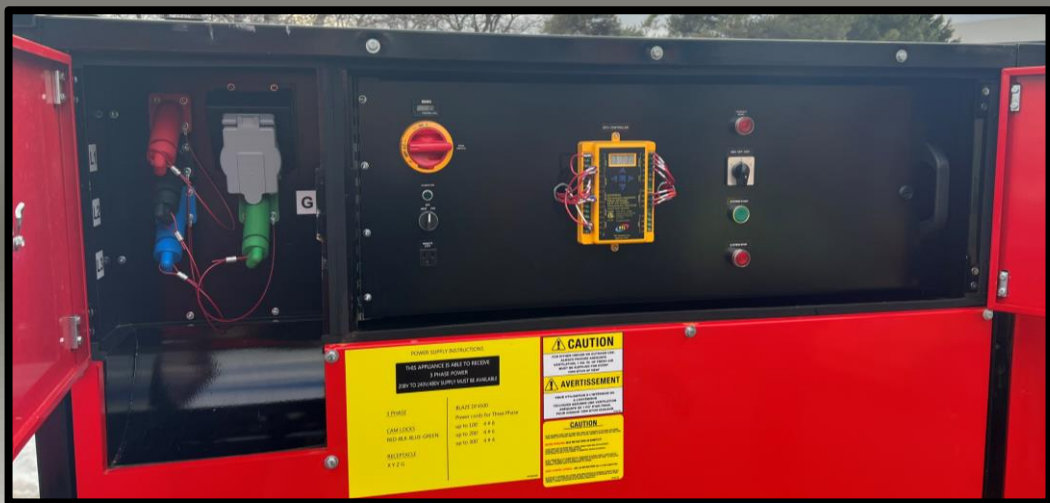
Dual Connections - Cam Locks or Twist, with Tamper Proof Door!
